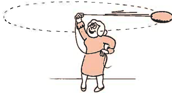
Fig. 11-11 An initially spherical ball of gooey taffy will be elongated when it is spun in a circular path.
