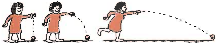
Fig. 12-1 The greater the stone's horizontal motion when released, the wider the arc of its curved path.
