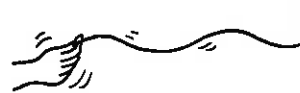
Fig. 25-5 When the string is shaken up and down, a disturbance moves along the length of the string.
