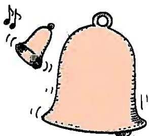
Fig. 26-9 The natural frequency of the smaller bell is higher than that of the big bell, and it rings at a higher pitch.
