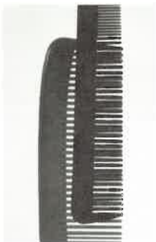
Fig. 26-16 The unequal spacings of the combs produce a moiré pattern that is similar to beats.
