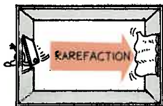
Fig. 26-4 (Top) When the door is opened, a condensation travels across the room. (Bottom) When the door is closed, a rarefaction travels across the room.
