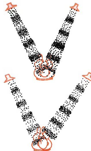
Fig. 26-14 Interference of sound waves. (Top) Waves arrive in phase. (Bottom) Waves arrive out of phase.
