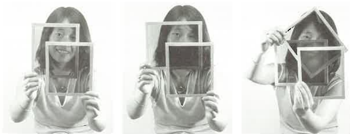
Fig. 27-20 Light is transmitted when the axes of the Polaroids are aligned (left), but absorbed when they are at right angles to each other (center). Interestingly enough, when a third Polaroid is sandwiched between the crossed Polaroids (right), light is transmitted. Why? (To answer, you'll have to know more about vectors. See Appendix C, Vector Applications.)
