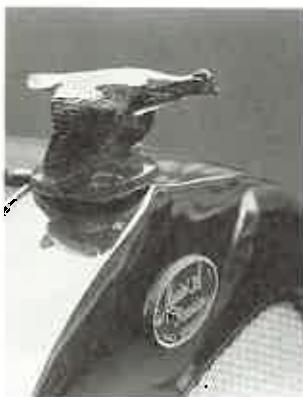
Fig. 27-10 Metals are shiny because light that shines on them forces free electrons into vibration. These electrons then emit their “own” light waves as a reflection.
