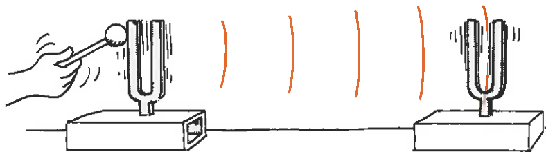
Fig. 27-6 Just as a sound wave can force a sound receiver into vibration, a light wave can force charged particles in materials into vibration.
