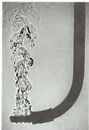
Fig. 27-15 A heater at the tip of the submerged J-tube produces convection currents in the water, which are revealed by shadows cast by light that is deflected differently by the water of different temperatures.
