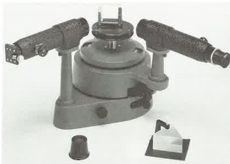
Fig. 28–16 A spectroscope. Light to be analyzed is placed near the thin slit at the left, where it is focused by lenses onto either a diffraction grating (shown) or a prism on the rotating table in the middle, and then viewed through the eyepiece on the right.
