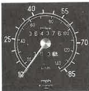
Fig. 2-2 The speedometer for a North American car gives readings of instantaneous speed in both mi/h and km/h. Odometers for the US market give readings in mi; those for the Canadian market give readings in km.
