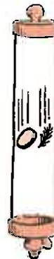
Fig. 2-8 A feather and a coin accelerate equally when there is no air around them.
