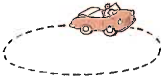
Fig. 2-3 The car on the circular track may have a constant speed, but not a constant velocity because its direction of motion is changing every instant.
