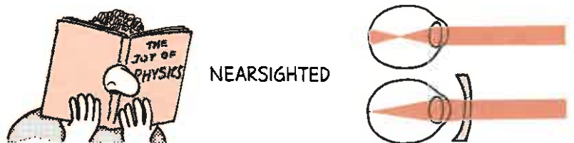
Fig. 30–22 The eyeball of the nearsighted eye is too long. A diverging lens moves the image farther away and onto the retina.
