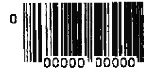
Fig. 31-25 A product's code is read by laser light that reflects from the bar pattern and is converted to an electrical signal that is fed into a computer. The signal is high when light is reflected from the white spaces and low when reflected from a dark bar.
