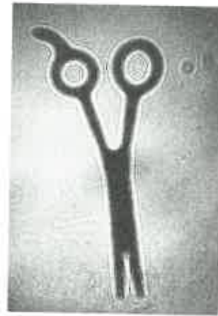
Fig. 31–8 Diffraction fringes are evident in the shadows of laser light, which is of a single frequency. These fringes would be filled in by multitudes of other fringes if the source were white light.
