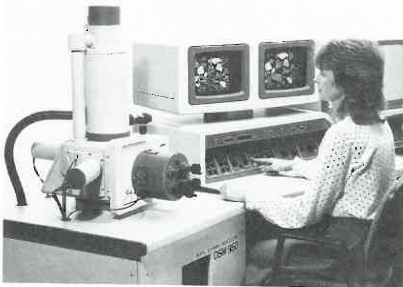
Fig. 31–9 Minimal diffraction by a very-short-wavelength electron beam in an electron microscope produces extraordinary detail.
