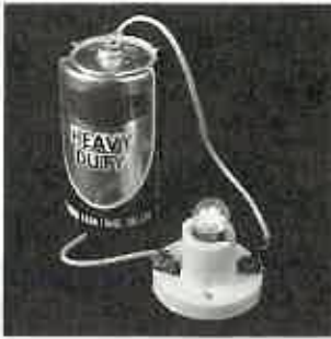
Fig. 34-3 Each coulomb of charge that is made to flow in a circuit that connects the ends of this 1.5-volt flashlight cell is energized with 1.5 joules.
