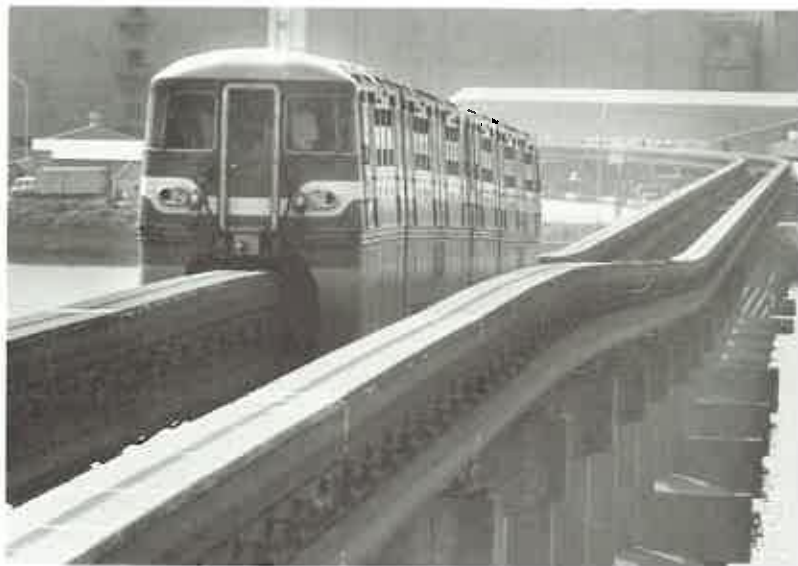
Fig. 36-14 Conventional trains vibrate as they ride on rails at high speeds. This Japanese magnetically levitated train is capable of vibration-free high speeds, even in excess of 200 km/h.
