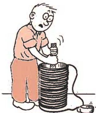
Fig. 37-4 It is more difficult to push the magnet into a coil with more loops because the magnetic field of each current loop resists the motion of the magnet.
