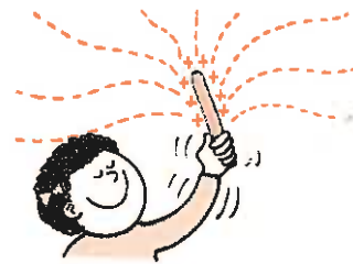
Fig. 37-16 Shake a charged object to and fro and you produce electromagnetic waves.
