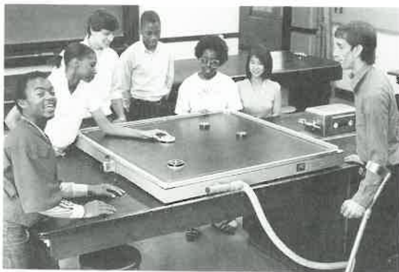
Fig. 3-5 An air table. Blasts of air from many tiny holes provide a friction-free surface.
