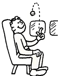
Fig. 3-12 Flip a coin in a high-speed airplane, and it behaves as if the plane were at rest. The coin keeps up with you: inertia in action.
