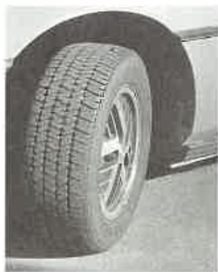
Fig. 4-11 Friction between the tire and the ground is the same whether the tire is wide or narrow. The purpose of the greater contact area is to reduce heating and wear.
