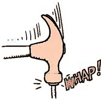
Fig. 5-2 The interaction that drives the nail is the same as the one that brings the hammer to a halt.
