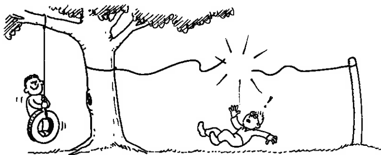
Fig. 6-7 You can safely hang from a piece of clothesline when it hangs vertically, but you'll break it if you attempt to make it support your weight when it is strung horizontally.
