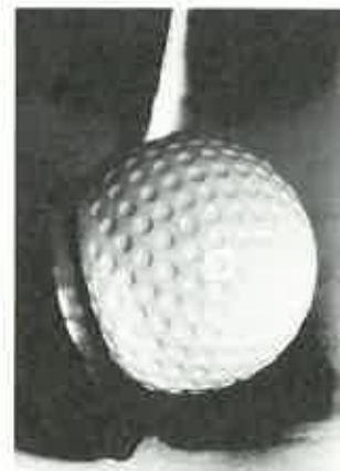
Fig. 7-2 The force of a golf club against a golf ball varies throughout the duration of impact.
