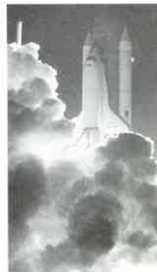
Fig. 8-2 The three main engines of a space shuttle can develop 33 000 MW of power when fuel is burned at the enormous rate of 3400 kg/s. This is like emptying an average-size swimming pool in 20 seconds!
