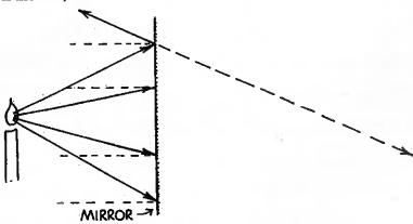
4. The ray diagram below shows the reflection of one of the rays that strikes the parabolic mirror. Notice that the law of reflection is obeyed, and the angle of incidence (from the normal, the dashed line) equals the angle of reflection (from the normal). Complete the diagram by drawing the reflected rays of the other three rays that are shown. (Do you see why parabolic mirrors are used in automobile headlights?)
