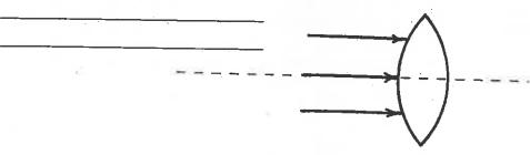
3. Show how light rays bend when they pass through the arrangement of glass blocks shown below.
