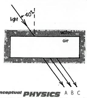
4. To the left, a light ray is shown moving from water into a rectangular block of air (inside a thin-walled plastic box), at 40° to the normal. Which of the three rays is most likely the light ray that continues into the water on the opposite side of the block?
